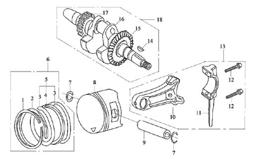
Note: When ordering parts from this list, specify: **Parts List D**, CRANKSHAFT, PISTON, AND CONNECTING ROD ASSEMBLY and the ITEM No.
